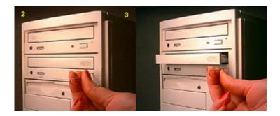
This procedure cannot be repeated without cycling the DVD-ROMs (computer's) power. After the media is removed and the loading tray is closed, the tray will not reopen without first turning the power ON/OFF.
